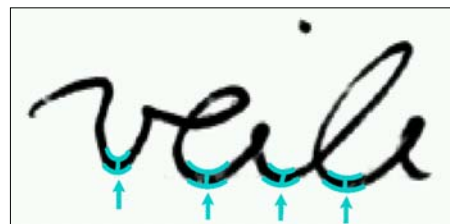
Figure 2. Segmentation at the minima in the lower contour that are proximal to the upper contour.
