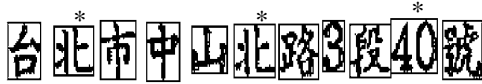
Figure 2. Character segmentation result. Characters marked with * are merged from two half-characters. The last one is merged erroneously.
