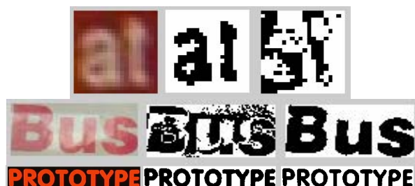
Figure 3: From left to right: initial image, clustering with ED and then with CS.
