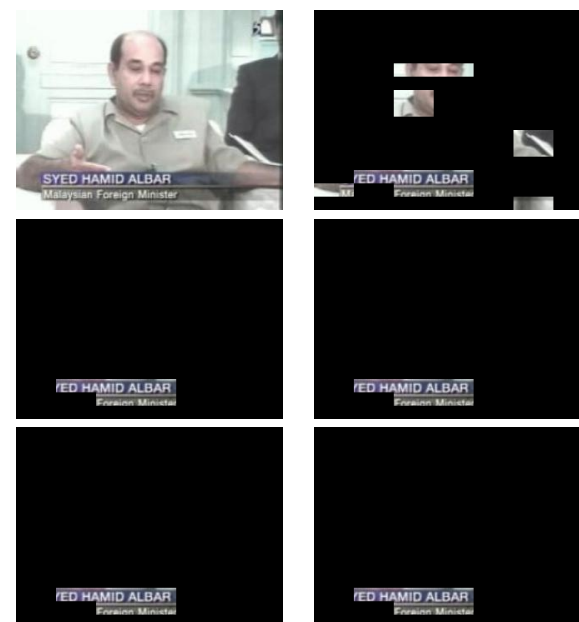
Figure 2. Results obtained with the sequential strategy (from left to right and top to bottom): original image, result from detector based on color, texture, edge density, edge regularity and final result.
