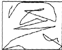
Figure 6. A single-stroke character created by connecting the 10 strokes of a character “ kindness” (“kindness”). This character was misrecognized as “ kindness” (“breath”) by \theta -HMM and correctly recognized as “ kindness” by (xy/\theta) -HMM.
