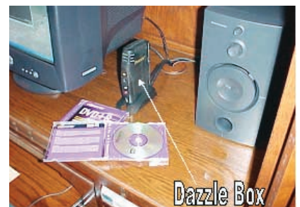
Figure 1. The Dazzle connection box. To transfer video clips to the PC, I connect the camcorder via Firewire cable to the Dazzle box that comes with Dell's Movie Studio bundle.
