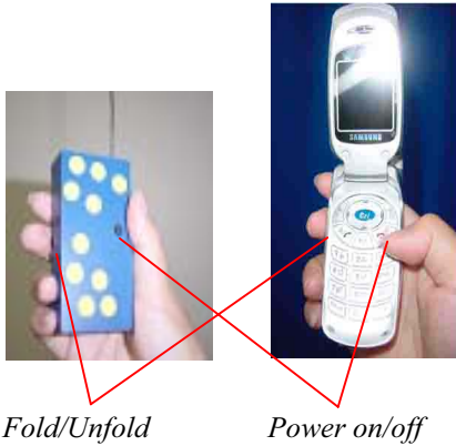
Figure 2. The prop used to replace actual mobile phones is simply a rectangular box with wireless event generating switches on them. The switches are wireless and sends push button events to the mother station through radio frequencies (the black line on top is the antenna), and the yellow dots on the prop are markers for camera tracking.
