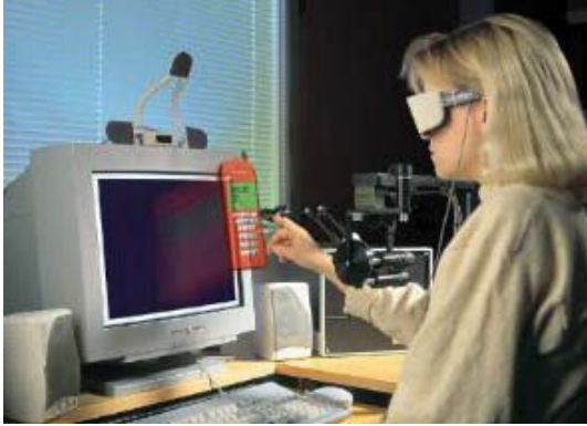
Figure 1. A desktop VR prototyping and evaluation system for mobile phones by researchers from VTT Electronics and University of Oulu, Finland [15]
