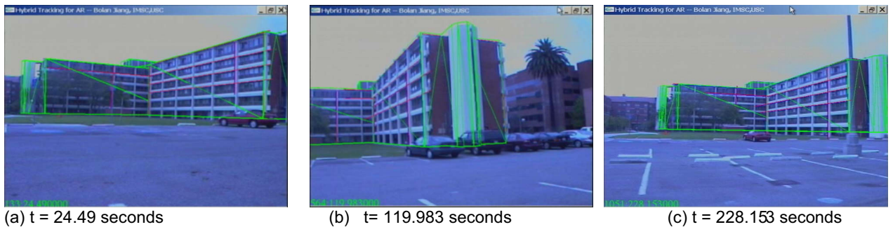
Figure 7 - Images from the first real-time tracking experiment. Green wire-frame model is the 3D augmentation. Red lines are the detected lines. Left-bottom corners have frame number: time stamp. Tracking sequence lasts about four minutes. (a) Tracking starts. (b) Middle of sequence. (c) Tracking continues successfully although a near-field pole occludes the building features.
