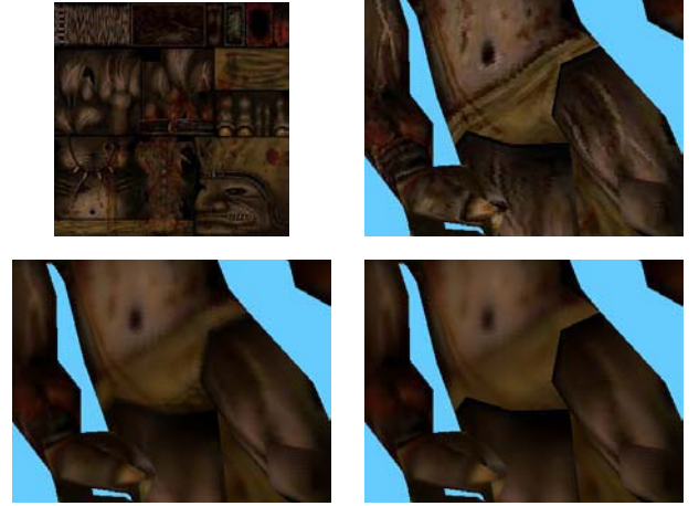
Figure 3: (top left) Original texture. (top right) Original model. (bottom left) Atlas-aware Laplacian smoothed with parameters \lambda = 0.25, n = 15 . (bottom right) Regular Laplacian smoothed texture using the same parameters. Notice the artifact at the hip.
