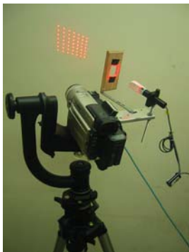
Figure 2 ModelCamera mounted in parallax-free pan-tilt bracket.
