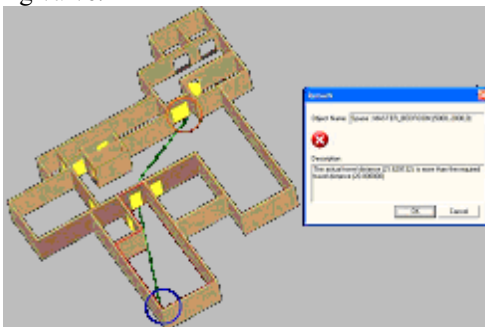
Figure 1. Visualization of the code checking result using the Code of Practice from FSB, Chapter 29, clause 2.2.2
