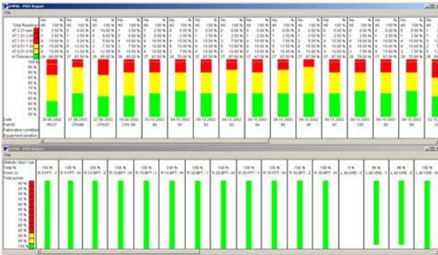
Figure 3: PIST (Point InSide Tolerance) analysis grouping either measurings or quality features
