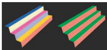
Figure 5. Face clustering methods: topologydriven methods (on the left) generate a cluster for each face, while octree quantisation correctly gives two clusters (clusters are shown in different colours - see colour plate).
