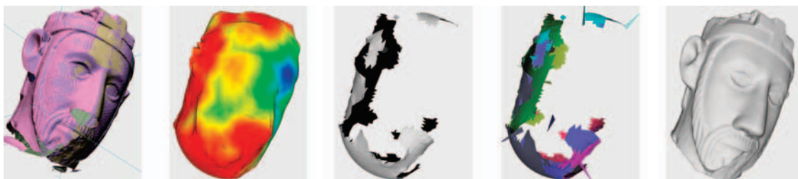
(a) Range maps before fusion and the resulting holefree mesh. The colour on the reconstructed surface maps the confidence value using the usual color ramp: red indicates surface portions that were acquired with a low confidence, are sampled in an insufficient way, or are associated to holes.
