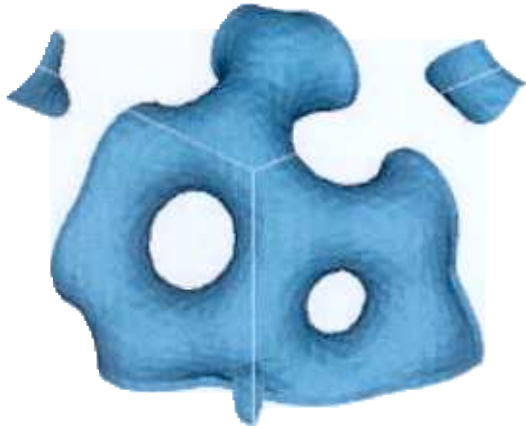
Figure 4. Uniform LOD extraction: error threshold equal to 0.1% of the field range. The isosurface for a field value equal to 105.000 is shown
