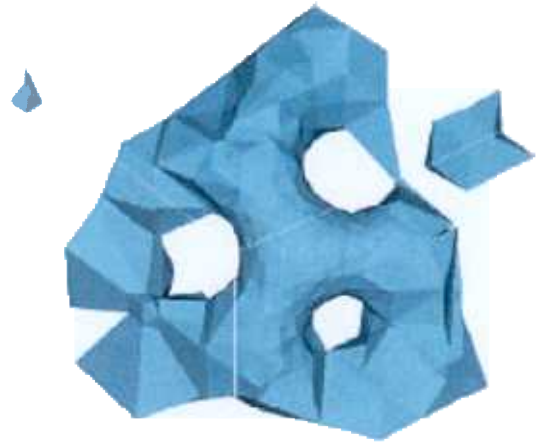
Figure 6. Variable LOD based on a region in space: mesh extracted with an error threshold equal to 0.1% of the field range in selected box, and arbitrary large outside. The isosurface for a field value equal to 105.000 is shown
