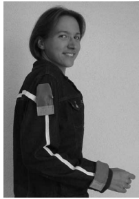
Figure 2. Usage of conductive textiles (white straps) to implement communication bus
