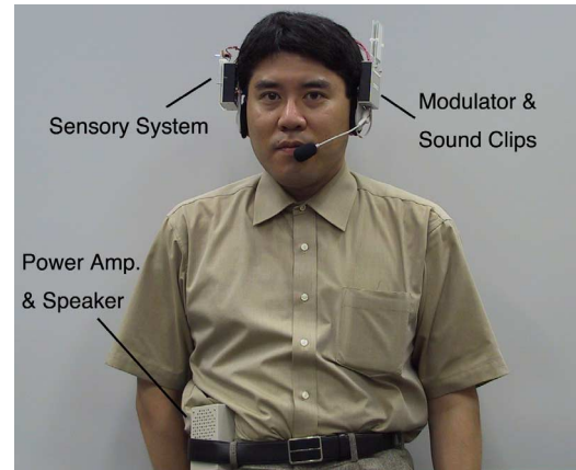
Figure 5. Setup example of the WCM system
