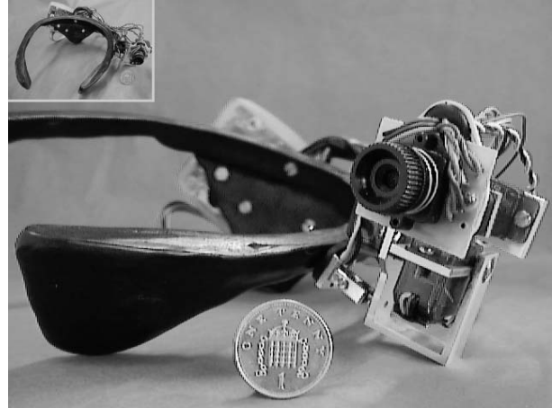
Figure 1. Collar-mounted wearable robot equipped with a miniature camera manipulated by a three-axis motorized active platform.
