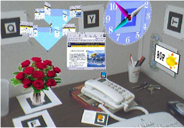
Figure 1. A typical ARWin desktop, as seen through a video see-through head-worn display (Sony LDI-A55 with Point Grey Firefly camera). Applications are (clockwise from right) weather report, tagged phone, business card, flowers, web browser, clock.
