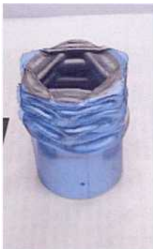
Figure 2: Augmentation of a crashed aluminum tube with the corresponding simulation results using a transparent visualization
