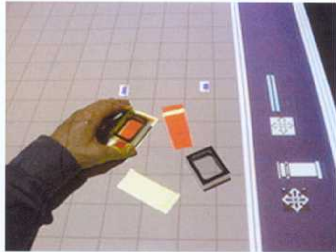
Figure 1: The TUI evaluated is called BUILD-IT. It offers a plan and a side view (left). The system is operated in the plan view using bricks (right).
