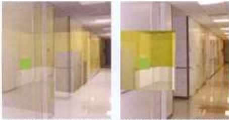
Figure 2: Sample solutions to depth ambiguity in an OIV/AR mockup. In these displays, the location of the rendered square is communicated more clearly by the use of transparency in these visualizations (compare to Figure 1). The use of transparent overlays (LEFT) conveys depth by letting the viewer see structure not otherwise visible, but while still perceiving the real-world structure. A similar approach (RIGHT) presents normally unseen structure by over-rendering a virtual “cut-away” of the occluding surfaces. This approach more clearly depicts the inside of the room, but at the cost of occluding real-world surfaces.
