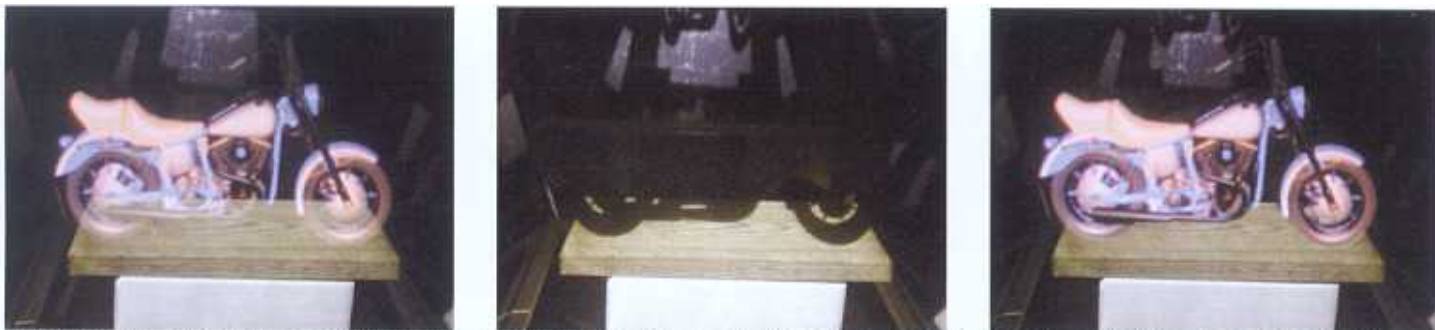
Figure 1. A normal illumination causes wrong occlusion effects between real objects and virtual overlays (left). Creating an occlusion shadow underneath the overlay prevents the light from being diffused on the real object's surface and transmitted through the optical combiner and the graphics (center). Overlaying the graphics over the shadow results in a realistic occlusion of the real object by the virtual one (left) 7 .
