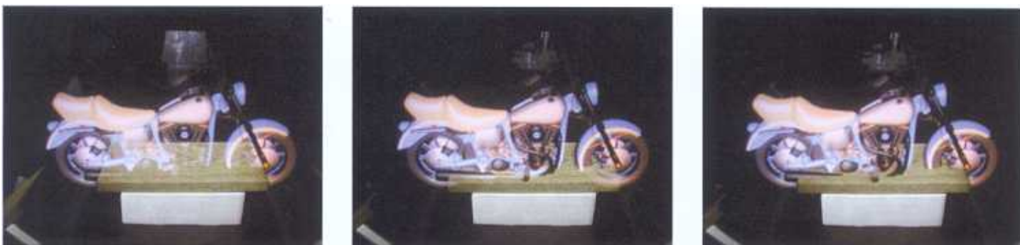
Figure 3. Knowing the depth information of the real content, also allows the occlusion of the virtual objects by the real ones (left). Combining this with our occlusion shadow method (center) creates correct mutual occlusion effects between both environments (right).
