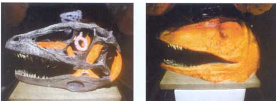
Figure 7. This example demonstrates our method in combination with a more complex real scene: A physical skull of a mid-cretaceous dinosaur (a Deinonychus) has been augmented with virtual muscles and bones (left) – generating occlusion shadows exactly underneath the virtual overlays. Covering the skull by a virtual skin (right) leaves most of the bone
