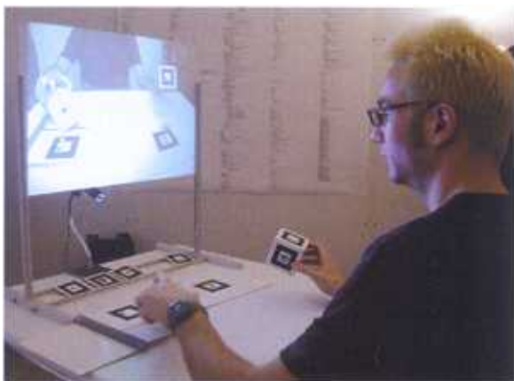
Figure 1. System set-up with a typical situation of use: charging the Gripper with an element from the booklet (left). The platform (right) holds an unsaturated atom, with which a binding with the charged atom may be triggered.
