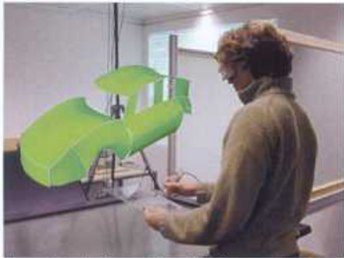
A car body is realized in Spacedesign using 3D devices and VR/AR visualization.
