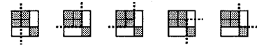
Figure 3: Illustration of the cuts which are not possible with a traditional one-point crossover.
