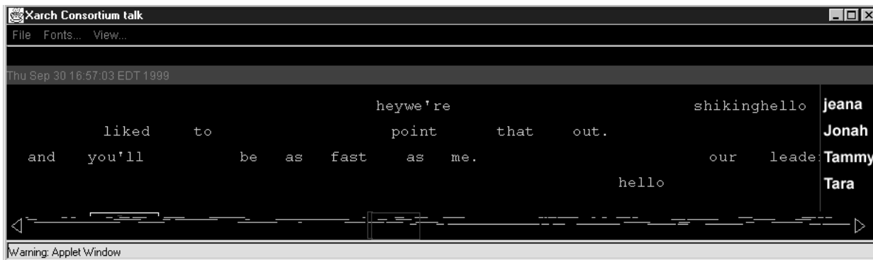
Figure 9. Fugue conversational window involves two main sections: the active conversation that can be read and moves along the horizontal, and the “zoomed out” view, or the iconic view, of the overall conversation. The iconic view acts as a navigation device to read the conversational history, as well as informs one about the kind of turn-taking patterns that have occurred.
