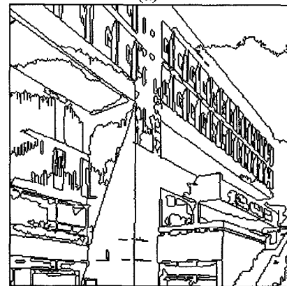
Figure 4. Gray level image segmentation. (a) Original, 256 \times 256 pixels. (b) Undersegmentation: 5 gray levels. Region boundaries.
