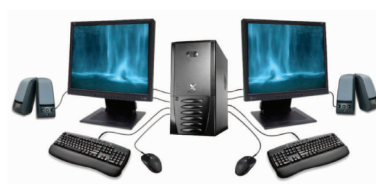
Open Sense Solutions' Groovix multiuser desktop in a single unit offers sound and 3D graphics to each user
